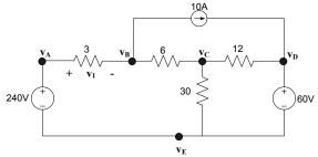
2. Pick a node and give it a known reference value. Keep things simple and make it a ground (zero volts).
