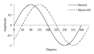
How do we write these two waveforms in polar form?
