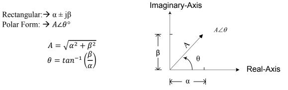
Note: for 2<sup>nd</sup> and 3<sup>rd</sup> quadrants an angle adjustment is required. Hence,
