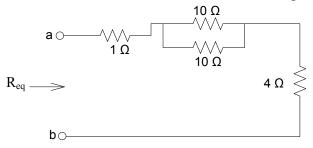
Therefore, equivalent resistance is now clearly seen as  $1\Omega$  in series with (10//10) in series with the  $4\Omega$ .
