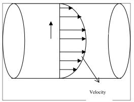
The velocity of water out of the pipe of inner radius 0.5 m, varies over the radial location in the pipe and is given below
