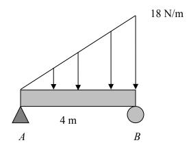
The beam is loaded as shown with a linearly distributed load. The beam is 4m long and its cross-sectional shape is  $0.2m \times 0.2m$  square. The Young's modulus of the beam is 210 GPa, and Poisson's ratio is 0.3. The reaction at point A is most nearly
