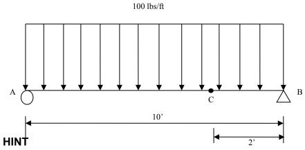
Find at least one of the support reactions. To do this reduce the distributed load to a concentrated load and apply equations of equilibrium.
