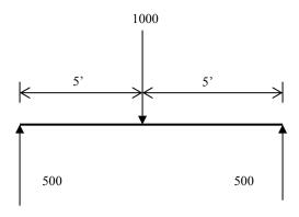
Note: Common mistake is to cut beam with distributed load reduced, in which case the answer is 500. However, this is wrong. You must cut beam at C, and then reduce the load. Looking at righthalf, we have:
